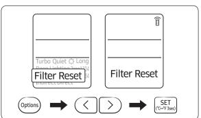
After cleaning and reassembling the air filter, be sure to reset the filter-cleaning reminder as follows:
